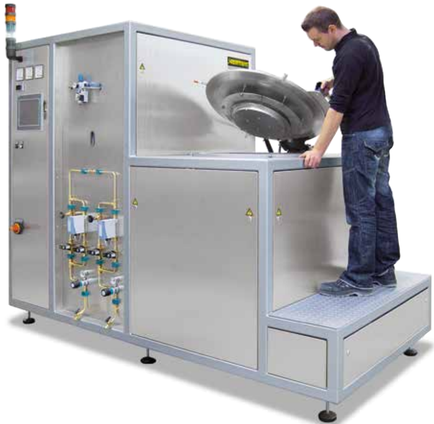
Retort furnace SVHT 9/24-W with tungsten heating
