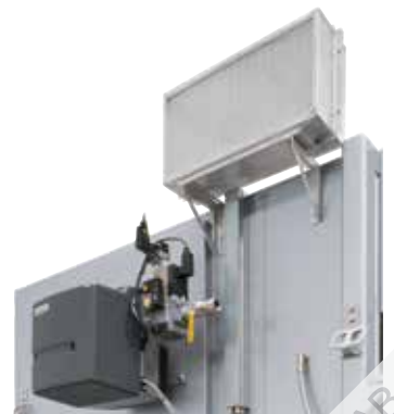
Direct gas-firing at a chamber dryer
