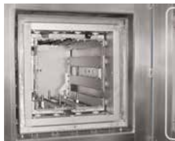
Molybdenum or tungsten heating chamber
