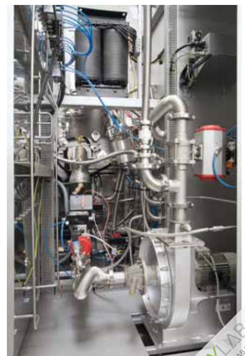
Rapid gas cooling, cold-wall retort furnace VHT 120-M
