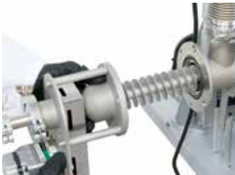
Screw-conveyor with adjustable speed
