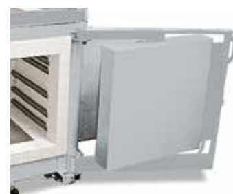
Parallel swinging door for opening when hot
