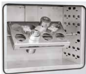
Electrical rotating device as additional equipment
