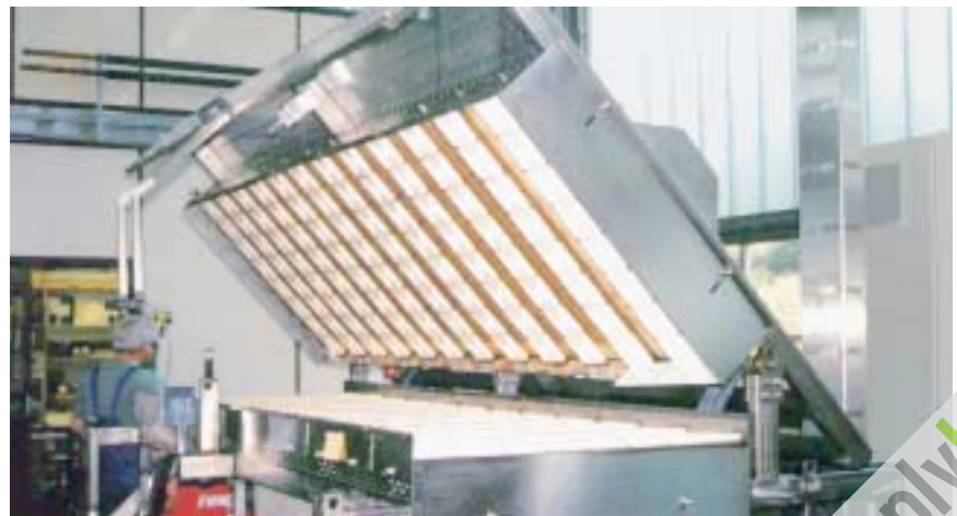
Heat treatment of glass fibre material prior to further processing
