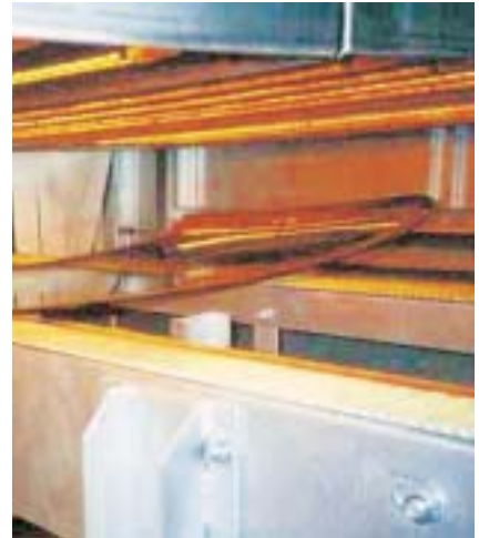
Heating the edges of automobile windows for improved PU foam retention
