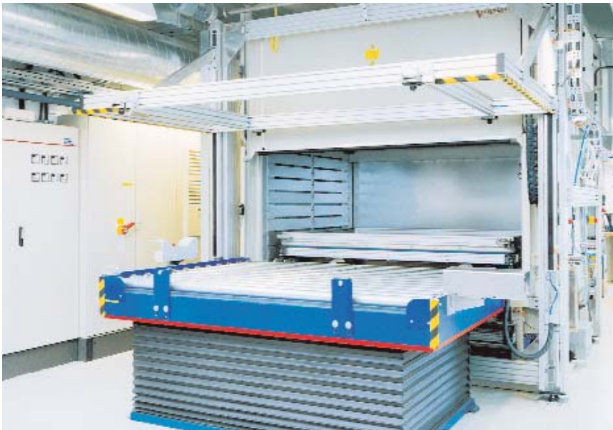
2-zone continuous oven for hardening carbon fibre composite material components
