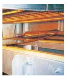
Heating the edges of automobile windows for improved PU foam retention
