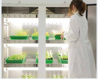
Reproducible, constant and uniform conditions for temperature, humidity and light are crucial for the quality of experiments. **fitotron**® SGC 120 Biological Chambers fulfil these requirements and also provide a high level of flexibility in changing test conditions.
